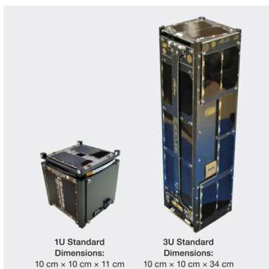
Figure 1. 1U CubeSat CP1 (left), 3U CubeSat CP10(right)[Cal Poly]
