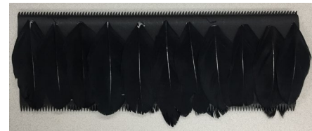
Fig. 6 Airfoil with serrations and feathers from the top views(H1)
