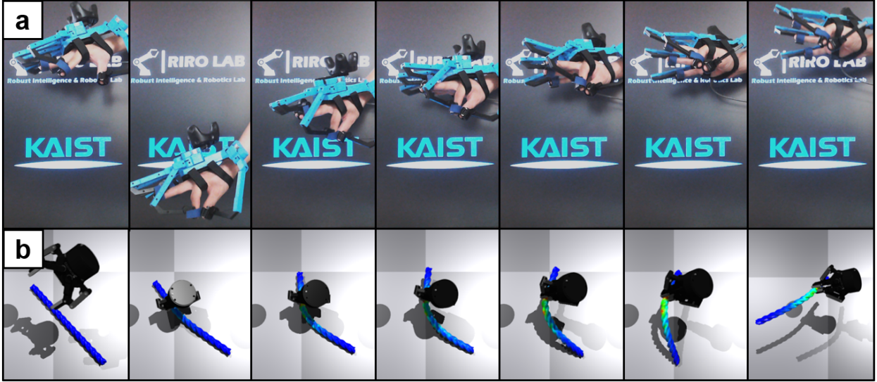
Fig. 4. Demonstration on the robot pick-up scenario, where a user virtually grasps the blue-color of simulated rope in IssacGym by observing its state via a 2D screen. In the simulation, the gripper is mounted on the invisible 6 DOF wrist robot.
